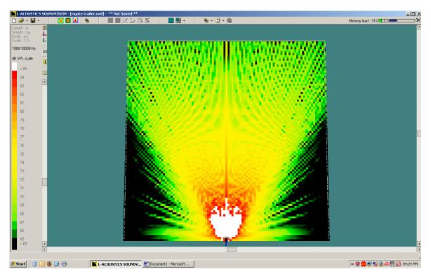
The stage is situated at the bottom of this picture, the model show that at 400m away in line (on axis) with the stage the sound level has dropped to 65dBA or below.
